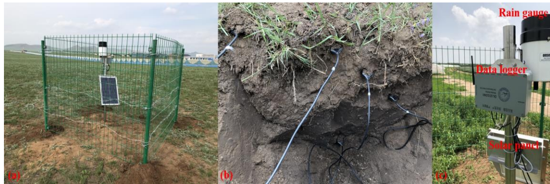
Figure 2. Installation of the in-situ measurement station, including a real photograph of the S2 station (a), a soil profile view when the 5TM sensor inserted (b), and installation of above-ground instruments (c).
