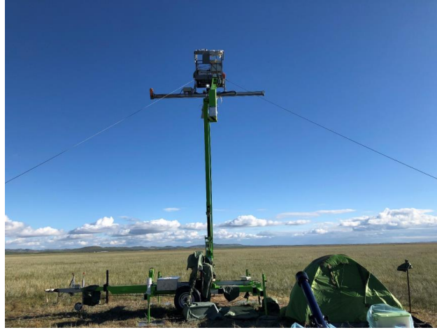
Fig. 2. The overview of GBSAR
