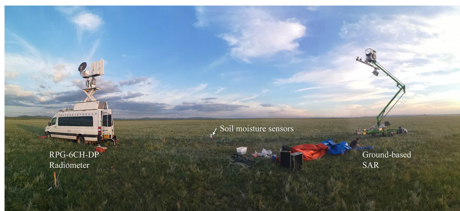
Fig. 5. Continuous observations of microwave emission and backscatter at a pasture site (Xinyuan).
